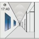
The light automatically turns on at 10% when natural light is insuffcient (no motion).
