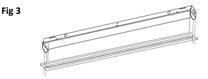
**Step 6**. A. If mounting to the 4 inch JBox, assemble the cover plates into fixture.
